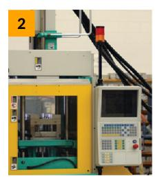
Plastic is injected into the mold, bonding with the in-mold label.
